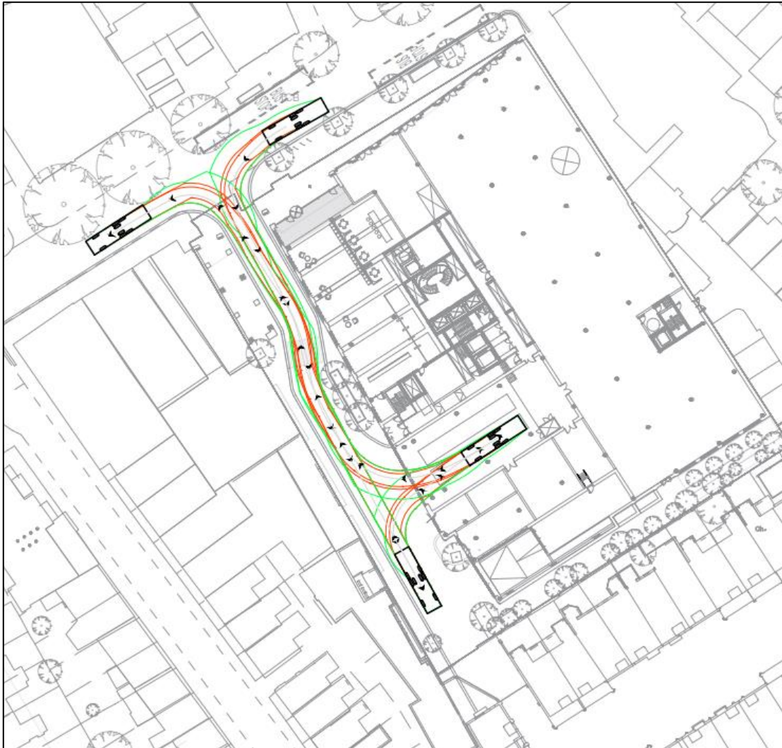
Extract from drawing no. 2204038-TK203 'Swept Path Analysis Refuse Vehicle', included as Appendix A of Operational Waste Management Plan, prepared by Motion ref. 2204038/paking dated 24/08/2023
